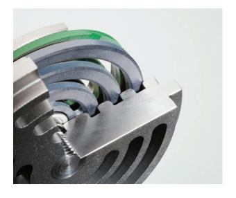
CP and CPs valves demonstrated a significant increase in reliability leading to extended service life as compared to valves with traditional design. The CP and CPs design implements new plate and seat port geometry along with a profiled sealing surface resulting in improved operating efficiency at a lower plate lift.
