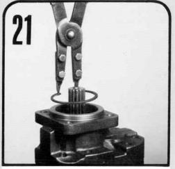
Install the snap ring in the groove.
