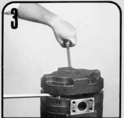
Lift off the port end cover. If necessary to pry loose, be careful not to damage the machined surfaces. Dowel pins will remain in either port end cover or gear housing. Do not remove. If the thrust plate remains in the gear housing, it can be tapped out later with a wooden hammer handle. Be careful not to distort the thrust plate.
