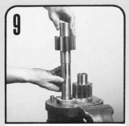
Insert the integral shaft and gear. Push down until the gear is tight against the thrust plate. Insert the matched driven gear.
