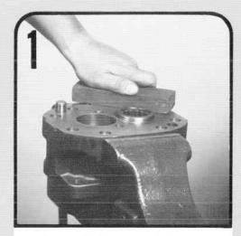
Stone off all cast machined surfaces with a medium grit carborundum stone (to remove any burrs as a result of disassembly). If bearings have been removed, deburr bearing bores. Rinse parts in a solvent. Air blast all parts and wipe with a clean, lintless cloth before starting reassembly.
