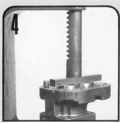
If any bearings have been removed from the shaft end cover, port end cover or bearing carrier, replace the bearings by pressing them into the bearing bore with an arbor press. Take care to avoid pressing on dowel pins.
