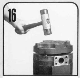
Place the port end cover over the gear journals and tap tightly against the gear housing. Be careful not to pinch the gasket seal.
