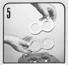
Check all thrust plates for wear. Replace if necessary (see below\*). Note that the thrust plates for pumps and motors can be different. Pump thrust plates, that have a single relief pocket must be installed with this pocket on the high pressure side. Motor thrust plates are grooved on both sides. The relief groove on all the unidirectional thrust plates must be towards the high pressure (outlet) side of the pump.
