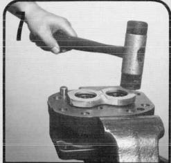
With the pocket seals down, place the thrust plate over the bearings. Tap thrust plate with a soft hammer to about 1/32" from the machined surface.
