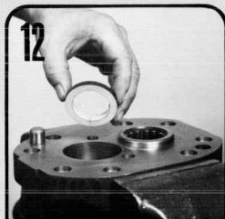
It is generally advisable to replace ring seals when rebuilding unit. To replace, remove the drive gear bearing with a bearing puller and remove ring seal from the bottom of bearing bore. Check all ring seal bores in unit for abnormal wear. If worn, replace those sections.
