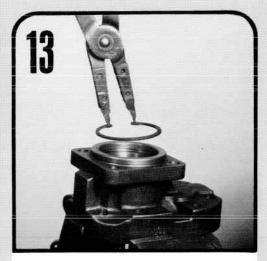
Grip the shaft end cover in the vise with the mounting face up. Remove the snap ring with snap ring pliers.
