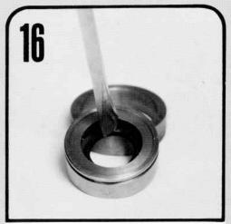
Tap the seal from the seal retainer and discard. Clean seal bore with solvent to remove old sealant. If bore is scored, smooth with fine grade emery paper. It is generally advisable to replace the seal retainer.
