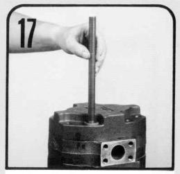
Thread the 8 fasteners (cap screws and washers, or studs and nuts) into the shaft end cover and snugup alternately or cross-corner. Rotate the drive shaft with a 6" wrench to make sure there is no binding in the pump.
