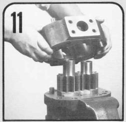
Slide the first section gear housing over the gears and tap it with a soft hammer until it rests tightly against the shaft end cover. Be careful not to pinch the gasket seal. Squirt oil over the gears to provide initial lubrication when pump is started.
