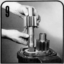
Remove the drive and driven gears. Keep the gears together because they are a matched set. Examine and replace if necessary. See pages 10 and 11.
