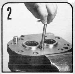
Grip the shaft end cover in the vise with the mounting face down. Examine the plug or 2 check valves, whichever is used, to be sure they are tightly in place. Replace only if parts are damaged or missing. Check valves can be removed with the special tool (see tool list). Screw in new valve with the tool until tight. Peen with a 1½" steel ball to secure.
