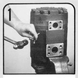
Place the pump in a vise with the drive shaft pointing down. Caution: DO NOT GRIP ON OR NEAR ANY MACHINED SURFACES DURING ASSEMBLY OR DISASSEMBLY. Index mark all sections with a punch. Be sure to align these marks when reassembling.
