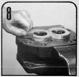
Cut 4 pocket seals approximately 7/16" long from the pocket seal strip. Insert one pocket seal into each of the slots in the thrust plate. Push each pocket seal all the way in so that they touch the roller bearings. Tap the thrust plate down firmly against the machined surface with a soft hammer. Use a sharp razor blade to trim exposed end of the pocket seal square and flush with the thrust plate.
