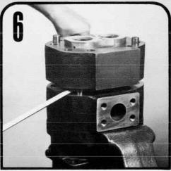
Lift or pry off the bearing carrier. Take care not to damage the machined surfaces.
