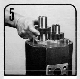
Remove the drive and driven gears. Keep the gears together because they are a matched set. Examine and replace if necessary. See below\*.
