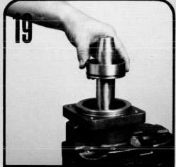
Grease and install the new "O" ring on the seal retainer. Lightly oil the installation sleeve and twist into the seal. Slide the sleeve over the drive shaft and push the seal retainer into place.
