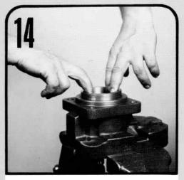
Remove the spacer or outboard bearing (pull the outboard bearing with a bearing puller).
