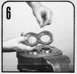
Cut 2 pocket seals 1-1/32" long from the pocket seal strip. Grease these pocket seals and insert into the middle slots in the thrust plate.
