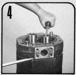
Lift the gear housing from the gears. If necessary to pry loose, take care not to damage machined surfaces.
