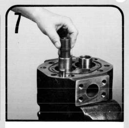
Remove the connecting shaft.
