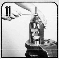
Examine all roller bearings for wear and discoloration. If replacement is necessary, pull the bearings with a bearing puller. Any sign of wear or discoloration calls for replacement. Remove bearings with a bearing puller.
