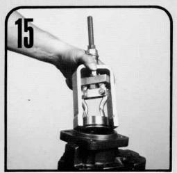
Remove the seal retainer and seal with a light duty bearing puller. Remove and discard "O" ring.
