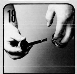
Coat the outside of the seal with Permatex Aviation Form-A-Gasket 3D or equivalent. With the metal side of the seal down, press it into the seal retainer with a 2¾" diameter bar and an arbor press. Be careful not to damage the lip of the seal.
