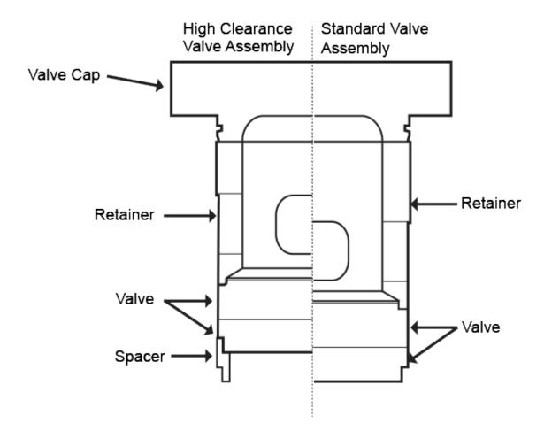
The cylinder DataBook lists the number of high clearance assemblies that can be provided with each cylinder and the percent of added fixed clearance for each assembly. A new cylinder purchased with high clearance assemblies will also be supplied with standard valve retainers.
