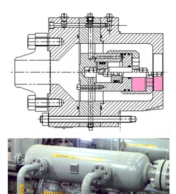
All deactivation configurations should be analyzed at all conditions to verify adequate rod load reversal.
