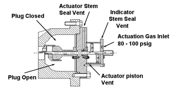
The FVCP requires 80-100 psi of air or gas pressure to operate. Actuation of the pocket can be performed by the PLC controlling a solenoid valve. In most cases, the FVCP is normally unloaded (FVCP open), requiring air or gas pressure to load (FVCP closed).
