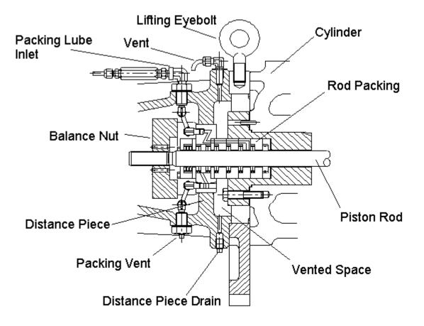
The short coupled distance piece is standard for the JGI, JGM, JGN, JGP, JGQ, JG, JGA, JGW, JGR and JGJ frames.
